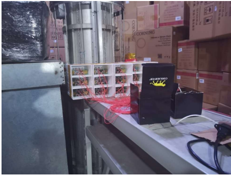
Figure 1 Device irradiation test
