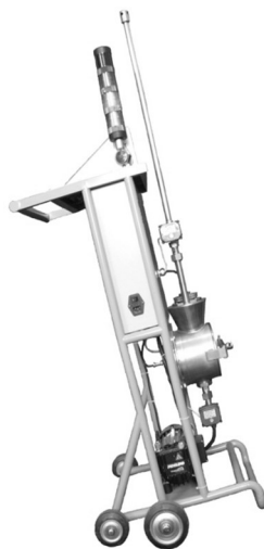
Figure 1 On - line New Type Artificial Nuclide Aerosol Monitor
