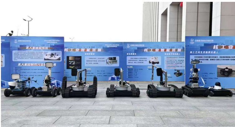
Figure 2 Small and Medium-Sized Robotic Platform System for Nuclear Emergencies and High-Radiation Scenarios
