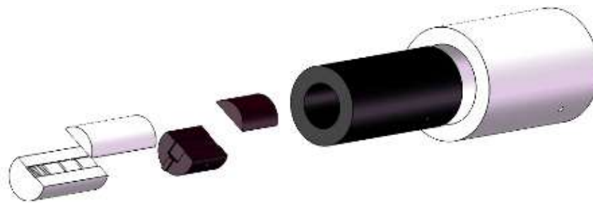
Fig.2. Schematic Diagram of the SNBS Moderator Structure (white part: polyethylene; black part: boron-doped polyethylene)
