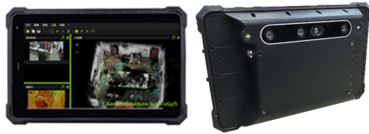
Figure 1 Instrument developed for VSLAM radiation based dose rate mapping
